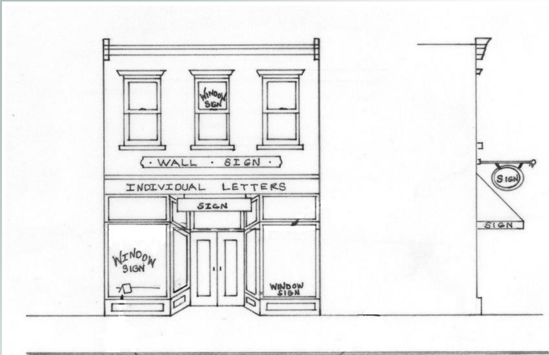
Shown above is appropriate signage placement on downtown commercial buildings.
